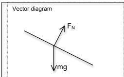
(a) Draw a vector diagram showing (and labelling) the forces acting on the car in the space indicated above.
