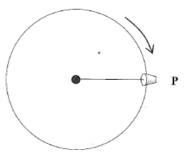
(a) If the rubber stopper completes a horizontal circle of radius 50.0 cm in 0.800 s, what is the magnitude of the tension in the fishing line?
