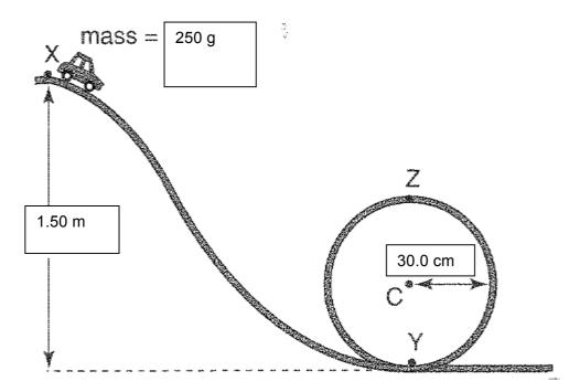
(a) Calculate the speed of the car as it reaches the bottom of the loop at point Y. (3 marks)
